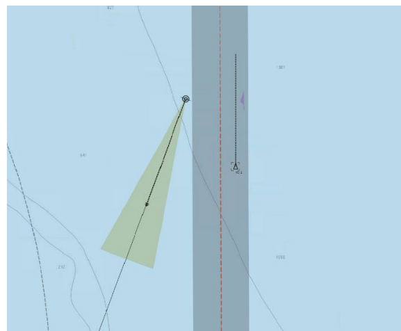
Ship manoeuvres outside the planned navigation corridor to avoid risk of collision
